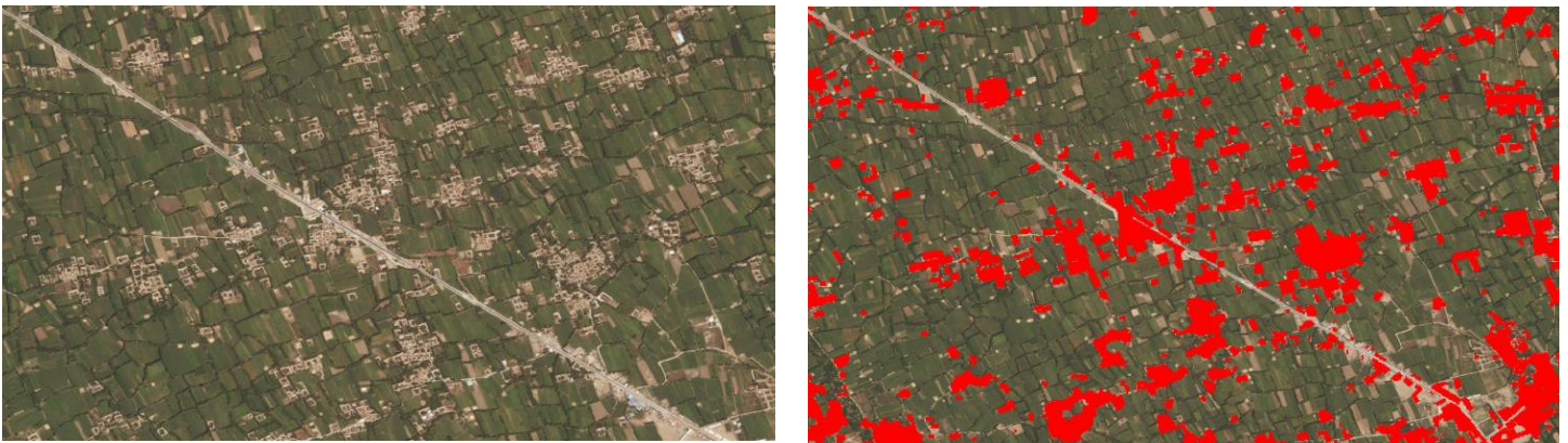
Figure 1: (left) High-resolution satellite image of a rural area of Afghanistan; (right) Settlement areas detected automatically by computer algorithms.
